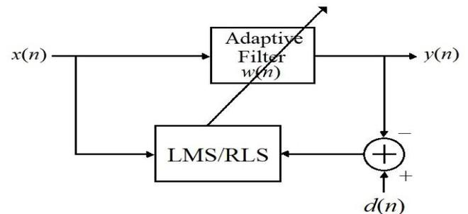
Figure 3. Block diagram for RLS adaptive equalizer
