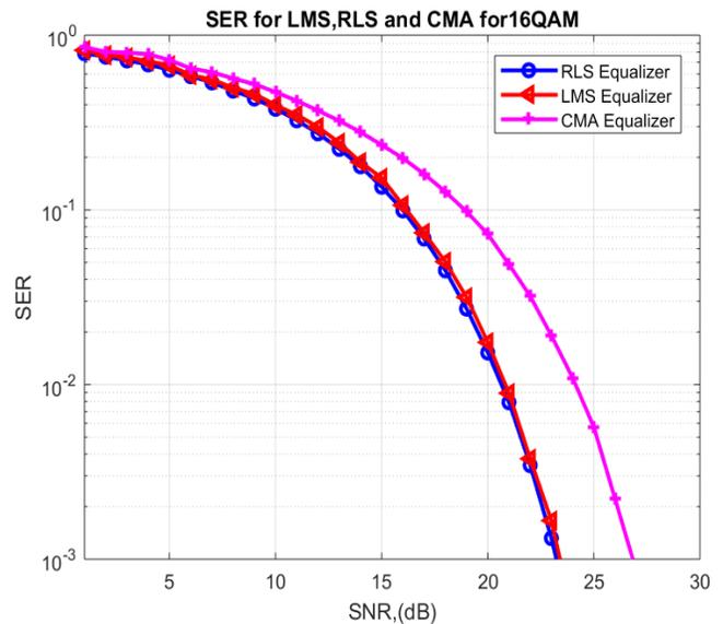
Figure 6: Results of RLS, LMS and CMA Equalization with 16-QAM
