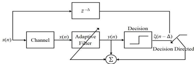
Figure 1: Digital transmission system using channel equalization
